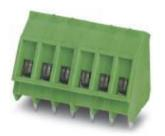
PCB terminal block, nominal current: 24 A, rated voltage (III/2): 400 V, nominal cross section: 2.5 mm², pitch: 5 mm, number of positions: 3, connection method: Screw connection with tension sleeve, mounting: Wave soldering, conductor/PCB connection direction: 55 °, color: green, Pin layout: Linear pinning, Solder pin [P]: 4.5 mm. The article can be aligned to create different nos. of positions!
