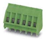
PCB terminal block, nominal current: 24 A, rated voltage (III/2): 400 V, nominal cross section: 2.5 mm², pitch: 5 mm, number of positions: 2, connection method: Screw connection with tension sleeve, mounting: Wave soldering, conductor/PCB connection direction: 55 °, color: green, Pin layout: Linear pinning, Solder pin [P]: 4.5 mm. The article can be aligned to create different nos. of positions!
