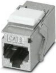
RJ45 socket insert, degree of protection: IP20, number of positions: 8, 1 Gbps, CAT6, material: Zinc die-cast, connection method: 2x RJ45, Keystone
