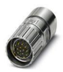
Cable connector, M23 PRO, straight, shielded: yes, Screw locking, M23, No. of pos.: 17, type of contact: Pin, Crimp connection, cable diameter range: 9 mm ... 15 mm
