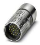
Cable connector, M23 PRO, straight, shielded: yes, ONECLICK fast locking system, M23, No. of pos.: 17, type of contact: Pin, Crimp connection, cable diameter range: 6 mm ... 10 mm
