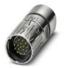
Cable connector, M23 PRO, straight, shielded: yes, ONECLICK fast locking system, M23, No. of pos.: 17, type of contact: Pin, Crimp connection, cable diameter range: 9 mm ... 15 mm
