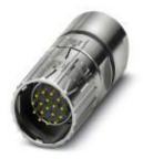
Cable connector, M23 PRO, straight, shielded: yes, ONECLICK fast locking system, M23, No. of pos.: 17, type of contact: Pin, Crimp connection, cable diameter range: 3 mm ... 15 mm
