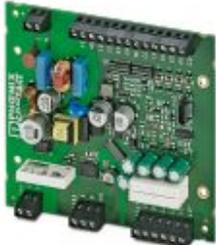
The EV-CC-AC1-M3-CBC-SER-PCB charging controller as PCB is used for charging electric vehicles at 3-phase AC networks according to IEC 61851-1, Mode 3. All charging functions, comprehensive configuration settings as well as a locking controller are already integrated.
