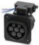
Socket Outlet, Rear protective cover screw connection, For charging electric vehicles (EV) with alternating current (AC), Compatible with infrastructure charging plugs, Type 2, IEC 62196-2, 32 A / 480 V (AC), Single wires, length: 0.7 m, Locking actuator: 12 V, 4-position, Rear panel mounting, Generation 1, "PHOENIX CONTACT" logo
