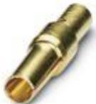
Crimp contact, turned, Single contact, contact diameter: 1 mm, crimp range: 0.5 mm<sup>2</sup> ... 1 mm<sup>2</sup>
