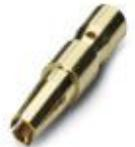
Crimp contact, turned, contact diameter: 1.5 mm, crimp range: 0.5 mm<sup>2</sup> ... 1 mm<sup>2</sup>
