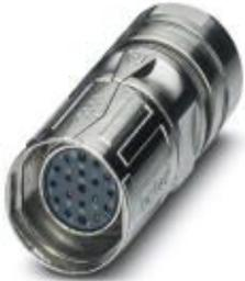
Cable connector, CA, straight, shielded: yes, SPEEDCON locking, M23, No. of pos.: 16+2+PE, type of contact: Socket, Crimp connection, cable diameter range: 10 mm ... 14.5 mm
