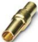
Crimp contact, turned, Single contact, contact diameter: 1 mm, crimp range: 0.14 mm<sup>2</sup> ... 0.56 mm<sup>2</sup>
