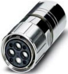
Cable connector, straight, Screw locking, M58, number of positions: 2+3+PE, type of contact: Socket, Crimp connection, shielded: yes, cable diameter range: 17 mm ... 25 mm
