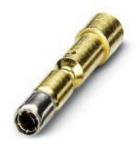
Crimp contact, Wire spring, Single contact, contact diameter: 1 mm, crimp range: 0.14 mm<sup>2</sup> ... 1 mm<sup>2</sup>
