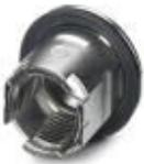
M12 threaded sleeve with tolerance-compensating function, for straight, THR solderable M12 socket contact inserts. Suitable for 2.4 mm ... 3.2 mm thick front plates.
