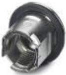
M12 threaded sleeve with tolerance-compensating function, for straight, THR solderable M12 socket contact inserts. Suitable for 3.1 mm ... 3.9 mm thick front plates.
