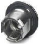
M12 threaded sleeve with tolerance-compensating function, for straight, THR solderable M12 socket contact inserts. Suitable for 1.7 mm ... 2.5 mm thick front plates.
