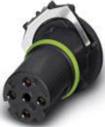
Bus system flat-type plug, Ethernet/PROFINET CAT5 (100 Mbps), 4-position, Socket, straight, D-coded, PCB mounting, THR solder connection
