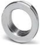
Reducing adapter, material: Brass, nickel-plated, connecting thread: M32 x 1.5, color: silver, with O-ring
