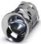
Metal screw connection with cable bend protection and strain relief, thread length: 8 mm, cable sealing area: 18 - 27 mm, clamping area: 20 - 30 mm, SW 40, screw connection: M32
