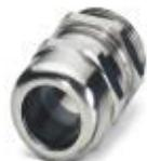
Cable gland, cable gland material: Nickel-plated brass, external cable diameter 15 mm ... 21 mm, shielding: no, connecting thread: M32 x 1.5, color: silver, with O-ring
