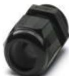
Cable gland, cable gland material: PA, external cable diameter 15 mm ... 21 mm, shielding: no, connecting thread: M32 x 1.5, color: jet black RAL 9005
