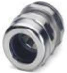
Cable gland, cable gland material: Nickel-plated brass, external cable diameter 14 mm ... 21 mm, shielding: yes, connecting thread: M32 x 1.5, color: silver, with O-ring
