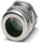
Metal screw connection up to 5 bar, thread length: 8 mm, cable diameter: 19 - 27 mm, WAF 43, screw connection: M32
