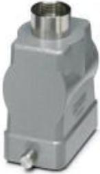
HEAVYCON sleeve housing B10, for single locking latch, height 72 mm, with support 1x M32, straight conductor exit
