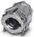
Metal screw connection with strain relief clamp, thread length: 8 mm, cable sealing area: 18 - 27 mm, clamping area: 19 - 30 mm, SW 40, screw connection: M32
