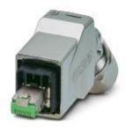
Push-pull connector (version 14), die-cast zinc, with RJ45 connector insert, 8-pos., with IDC fast connection technology, for 1 and 7-wire cores, 23 ... 22 AWG, for cable diameter of 5.5 mm ... 10 mm
