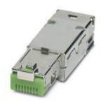
Contact insert, degree of protection: IP20, number of positions: 8, 1 Gbps, CAT5 (IEC 11801:2002), material: Zinc die-cast, connection method: IDC fast connection, connection cross section: AWG 26-24, cable outlet: straight
