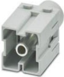
Contact insert module, number of positions: 1, power contacts: 1, control contacts: 0, Pin, Axial screw connection, 1000 V, 200 A, 25 mm<sup>2</sup> ... 70 mm<sup>2</sup>, application: Power
