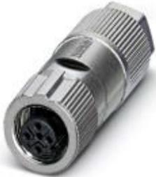
Bus system connector, PROFIBUS DP (12 Mbps), 2-position, halogen-free, shielded, Socket straight M12 SPEEDCON, Coding: B, Insulation displacement connection, knurl material: Zinc die-cast, nickel-plated, external cable diameter 5 mm ... 9.7 mm
