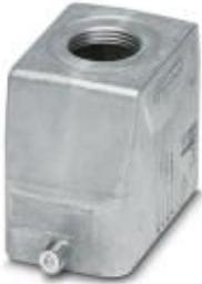
Sleeve housing B10, for single locking latch, material: Die-cast aluminum, salt water resistant, cable outlets: 1, straight, height: 57 mm, cable gland: none, support sleeve: no, 1x M25, Standard
