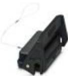
Protective cover B10, with single locking latch, protective cover material: PA, height: 21.6 mm, seal: yes, diameter of retaining cord eyelet: 30 mm
