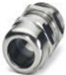
Cable gland, cable gland material: Nickel-plated brass, external cable diameter 11 mm ... 17 mm, shielding: no, connecting thread: M25 x 1.5, color: silver, with O-ring
