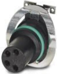
Flush-type connector, 4-position, Socket, straight, M8, A-coded, PCB mounting, SMD
