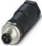
Power connectors, Power, 4-position, unshielded, Plug straight M12, Coding: T, Screw connection, knurl material: Zinc die-cast, nickel-plated, cable gland Pg11, external cable diameter 8 mm ... 10 mm, For direct current up to 12 A/63 V, Contact 4 leading
