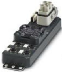
Power distributor, application: Power supply, connection method: M12 socket Metal, number of slots: 4, number of positions: 4, coding: T power, slot assignment: single, status display: yes, Universal; master cable connection: Plug-in master cable connection 90°, shielding: no, Diagnostics port, M12, A-coded, 12-pos.
