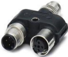
Y distributor, Ethernet hybrid CAT5 (100 Mbps), 8-position, shielded, Plug straight M12, coding: Y, on Socket straight M12, coding: D and Plug straight M12, coding: A, Power with Ethernet (PWE), Thread M12 plug A-coded and M12 socket not rotatable
