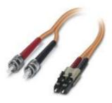
Assembled FO cable, zip cord cable, multi-mode fiberglass 50/125  $\mu$ m, OM2, plug: LC/B-FOC (ST), degree of protection: IP20, for installation in cable ducts or control cabinets, length: 1 m
