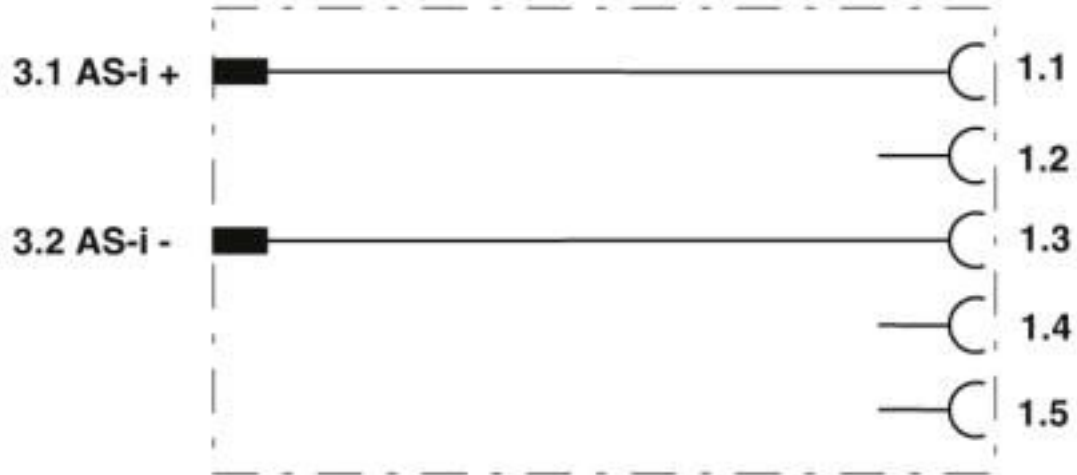
Contact assignment of the AS-Interface distributor
