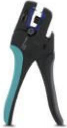
Stripping tool, laser marked according to customer specifications, for cables and conductors from 0.02 - 10 mm<sup>2</sup>, self-adjusting, stripping length of up to 18 mm, cutting capacity of up to 10 mm<sup>2</sup> stranded/1.5 mm<sup>2</sup> solid, replaceable stripping blade
