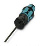
Torque screw driver with preset torque of 0.8 Nm, with 4 mm hexagon for accommodating SAC bits, two-component handle with non-slip grip
